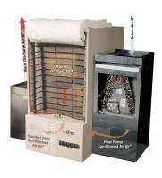
within special, **high-density ceramic bricks.** When the thermostat asks for heat, the ETS unit sends the home's return air through the heated ceramic bricks and further sends the warm air into the home's living areas.
